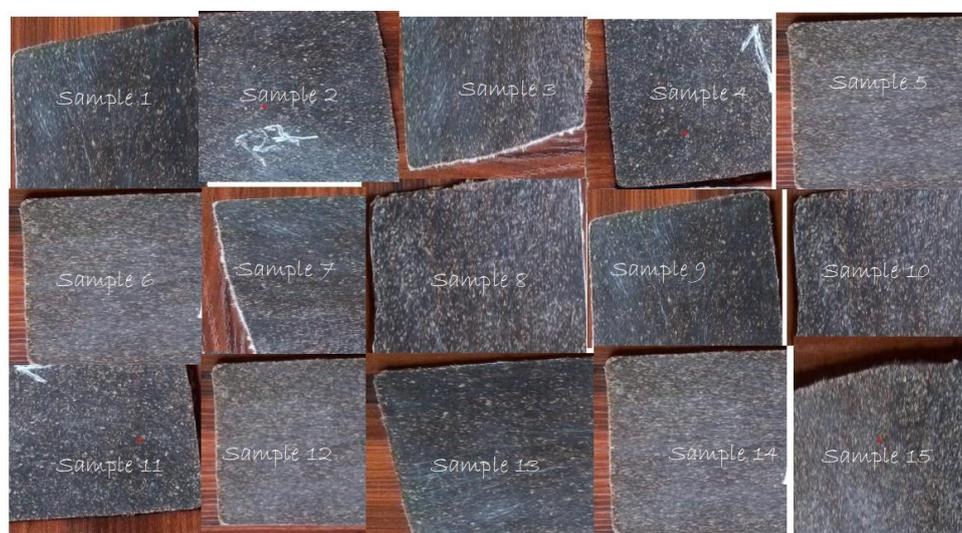
**Figure 5.** Rice husk-based reinforced particle board.
