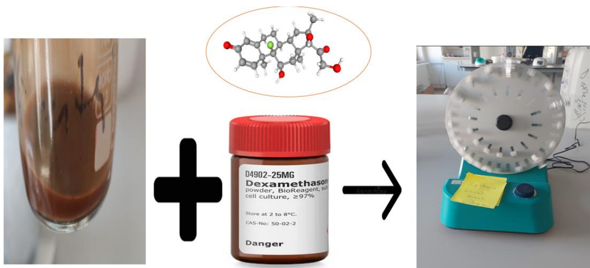
Figure 2. Drug loading analyses. The drug was loaded onto free magnetic nanoparticles by stirring at room temperature for 24 h using a rotator machine.
