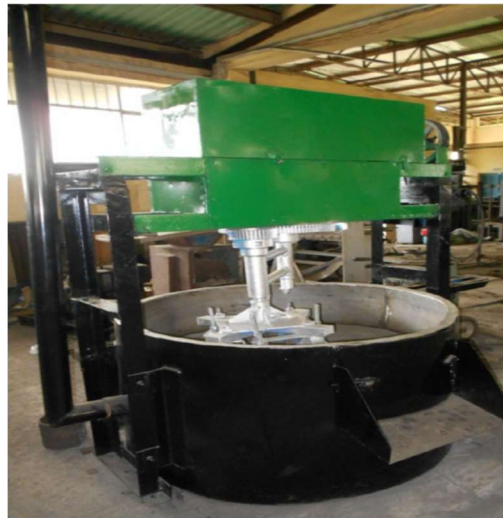
Figure 5. NCAM developed mechanical gari fryer.
