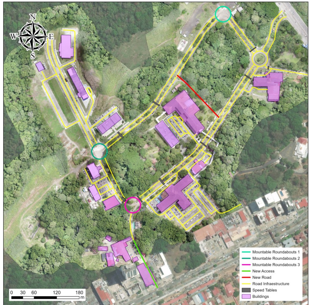
Figure 6. Location of the improvement simulated for driving safety within the UTP VLS Campus.
