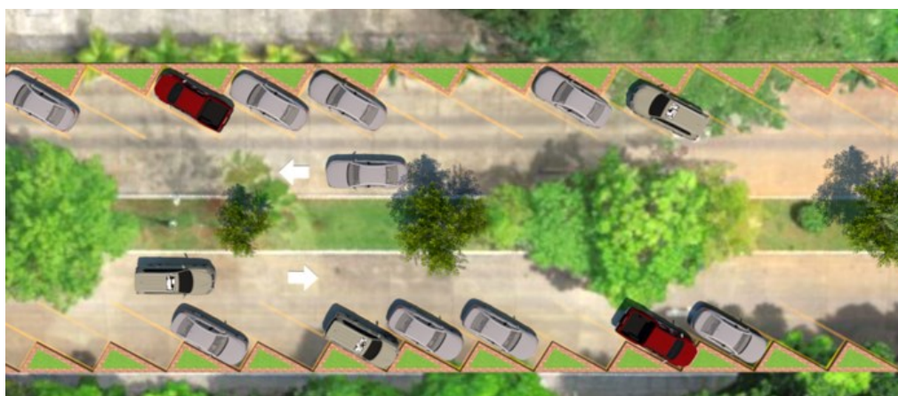
Figure 10. Plan-view showing the improvements included in the parking lot simulation at a 30-degree angle.
