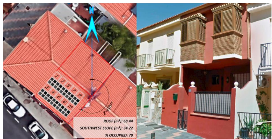
Figure 2. Floor plan and view of the dwelling in Malaga. Ten solar panels (the maximum possible number) occupy 70% of the surface area (34.22 m 2 ) of the southwest-facing roof slope, while the remaining 30% is reserved for maintenance purposes (Source (images): Google Earth).
