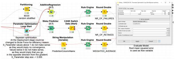
Figure 2. The settings of Hyper-Parameter Optimization loop for BART forecasting method.
