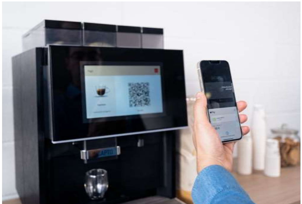
Figure 10. Every machine is connected and coffee can be paid and delivered through QR identification and every mobile payment method.
