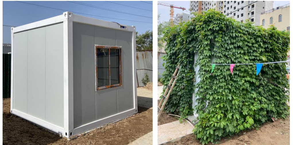
Figure 1. Experiment room (a) Reference room; (b) Indirect green façade room.
