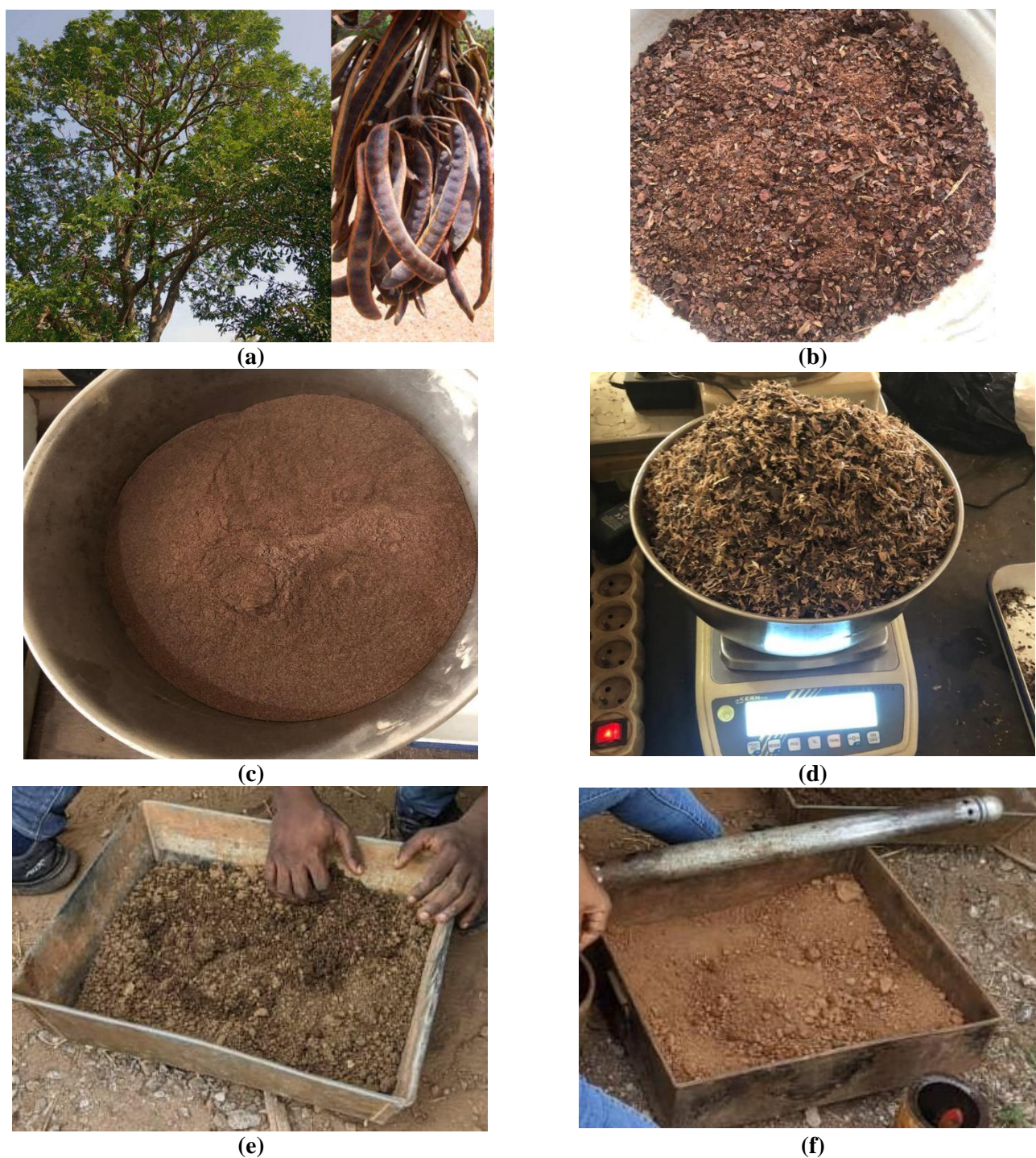
Figure 1. The materials used, (a) African locust bean tree and pods; (b) African locust bean pod powder passing 2 mm; (c) African locust bean pod powder, passing 0.08 mm; (d) African locust bean pod powder with a diameter between 2 mm and 5 mm; (e) soil from Tsévié; (f) soil from Soumdina.
