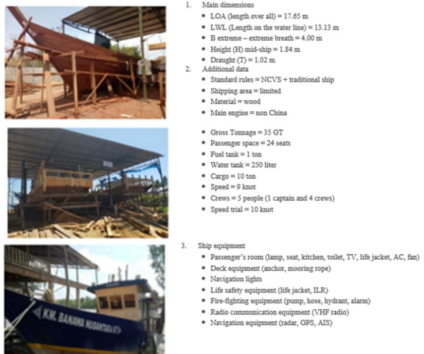
Figure 6. Technical specifications of the traditional shipping grant vessels.
