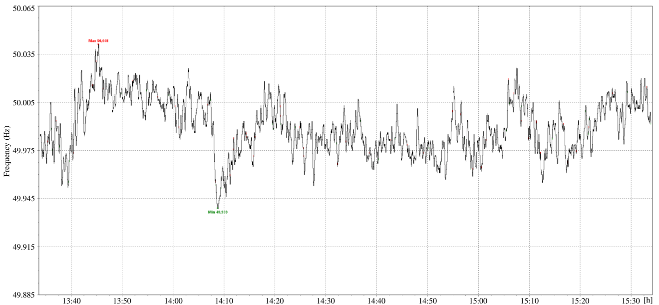
Figure 14. Frequency variation mode of the voltage supplied by the 60 kW PV system.
