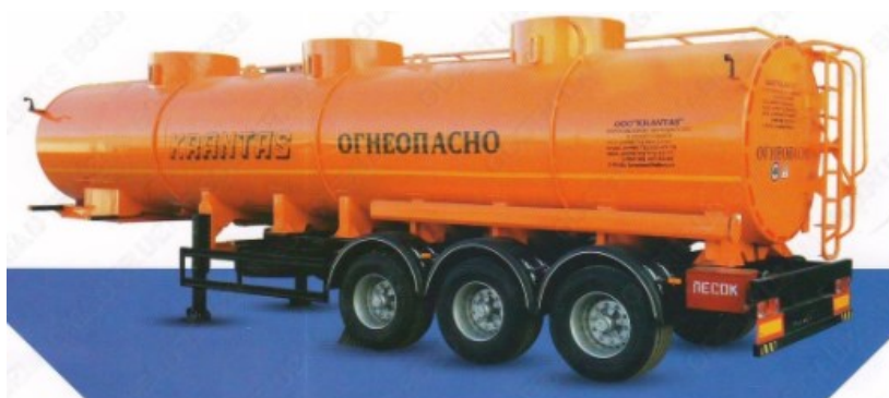
Figure 1. KRANTAS Petrol trailers already used by the company (capable of transporting 22.5 tones of different types of petrol and diesel fuel in 3 compartments).
