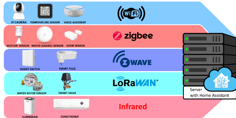
Figure 3. Architecture of multi-layer integration of wireless protocols.
