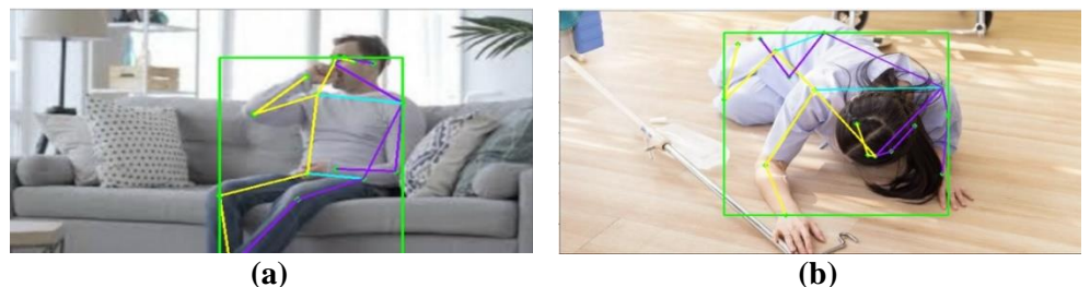
Figure 5. Samples of dataset. (a) Example of a “Not Fall” class with keypoints illustrated; (b) example of a “Fall” class with keypoints illustrated.
