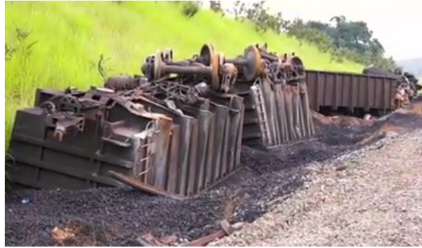
Figure 4. Deraiment of an ore train in 2019.
