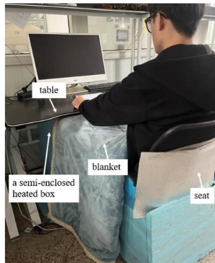
**Figure 1.** Blanket installation diagram.
