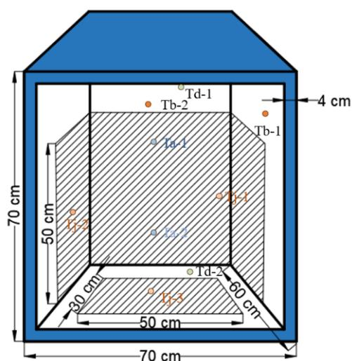
**Figure 4.** Layout of temperature measurement points inside the heated box.
