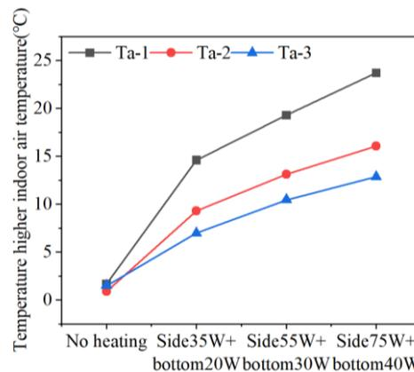
**Figure 9.** The air temperature inside the box when the indoor temperature was about 10 °C.
