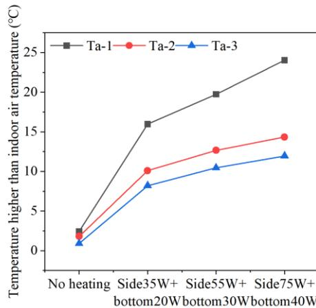
**Figure 12.** The air temperature inside the box when the indoor temperature was about 8 °C.
