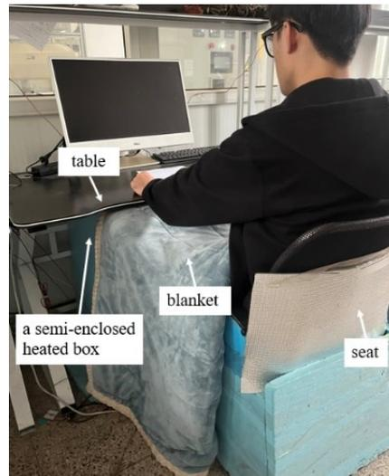
**Figure 1.** Blanket installation diagram.
