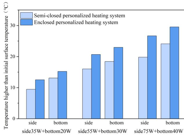
**Figure 6.** The surface temperature of the heated film higher than that of the initial no-heating condition under different heating powers.
