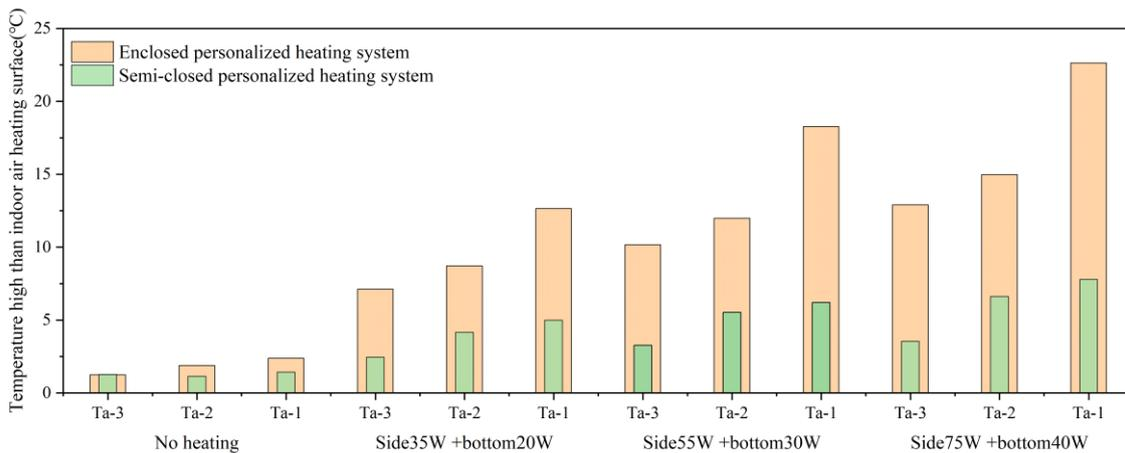
**Figure 7.** The air temperature inside the box (Ta-1, Ta-2) and under the seat (Ta-3) higher than the indoor ambient temperature (12 °C).
