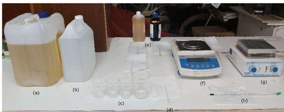
**Figure 3.** (a) laboratory equipment and material-diesel fuel; (b) deionised water; (c) beakers; (d) pipette; (e) surfactants; (f) analytic balance; (g) magnetic stirrer; and (h) thermometer.
