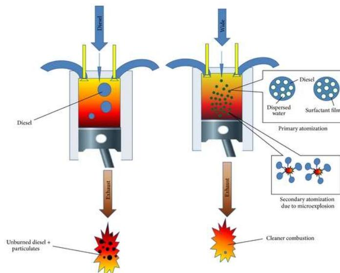
**Figure 1.** Primary and secondary atomization of WiDE [15].
