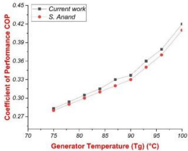
**Figure 9.** Comparison of COP of current work with the work of Anand [13].
