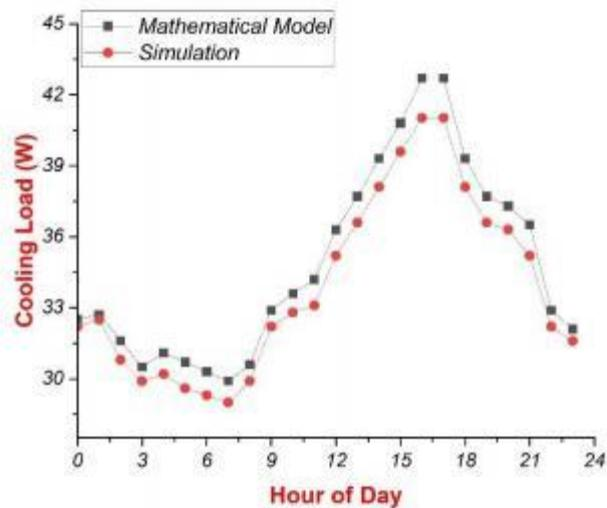
Figure 8. Comparison of mathematical model and HAP simulation for cooling load.
