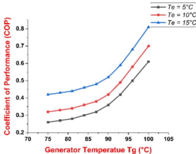
**Figure 10.** Variation of COP with generator temperature at different evaporator temperatures ( $T_c = 30\text{ }^\circ\text{C}$ ).
