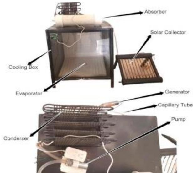
**Figure 6.** Complete experimental setup.
