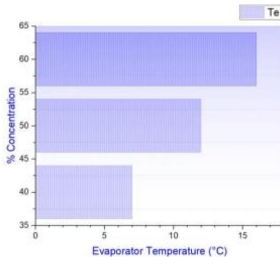
**Figure 12.** Variation of maximum temperature drop of evaporator.
