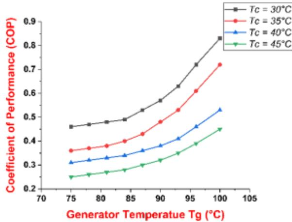
**Figure 11.** Variation of COP with generator temperature at different condenser temperatures ( $T_e = 5^\circ\text{C}$ ).
