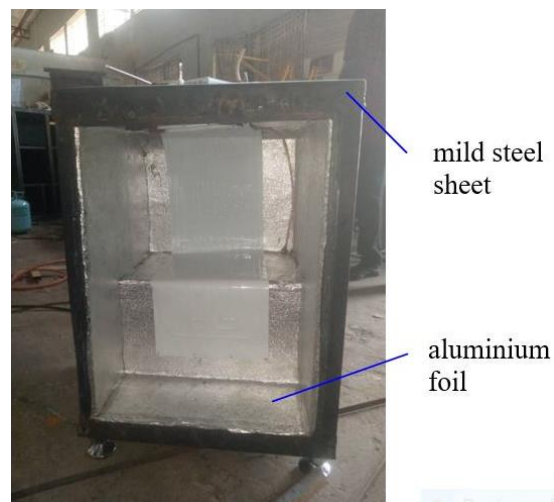
Figure 3. The laying of the walls of the refrigerator.
