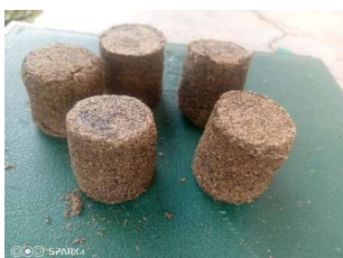
Figure 5. Image of fuel briquette from mixture of cattle manure and sawdust.
