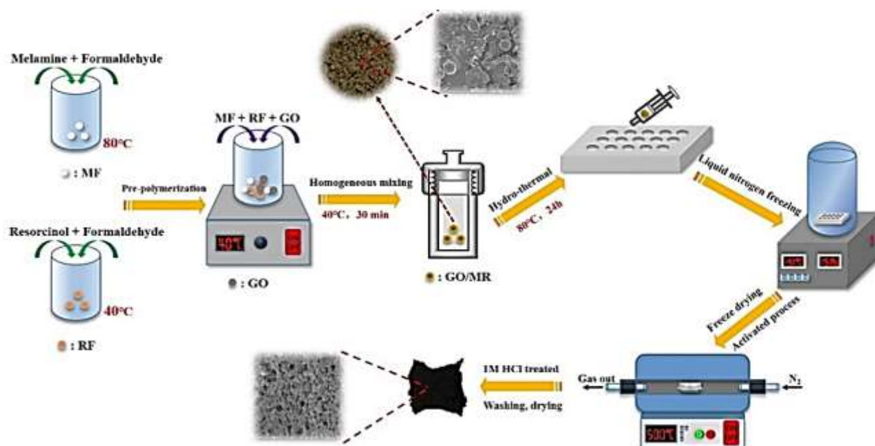
Figure 1. Schematic exhibition of hydrothermal synthesis process for N-doped activated carbon materials derived from a GO/MR composite. Reproduced by permission from Ref [30].
