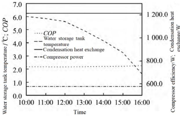
Figure 9. Variation of the performance of heat pump system.
