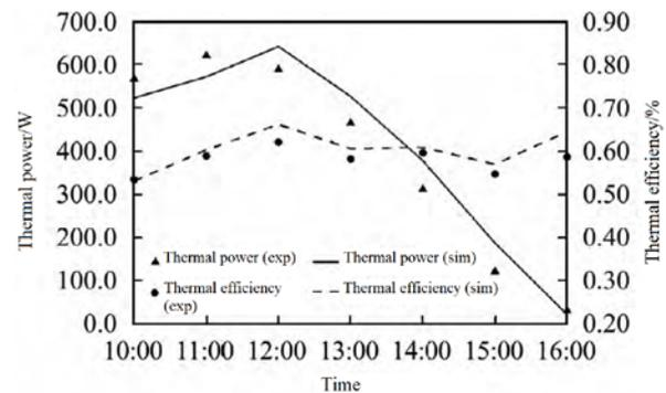
**Figure 4.** Comparison of measured and simulated values of thermal performance.
