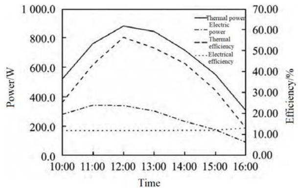
Figure 10. Variation of thermoelectric performance after optimization.
