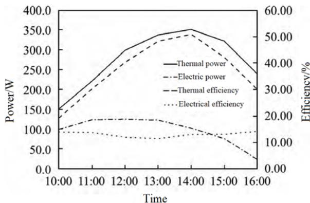
**Figure 8.** Variation of the thermoelectric performance.
