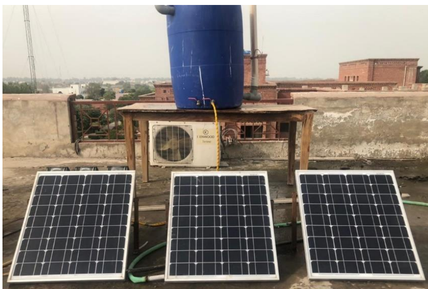
Figure 2. Experimental setup for simple PV modules and modules with cooling techniques.
