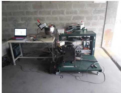
Figure 11. Engine bench-test of the emulsion.
