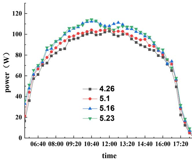
**Figure 8.** The power output curves of the passive sun-tracking system at various sunny days in the spring season showing the temperature effect.
