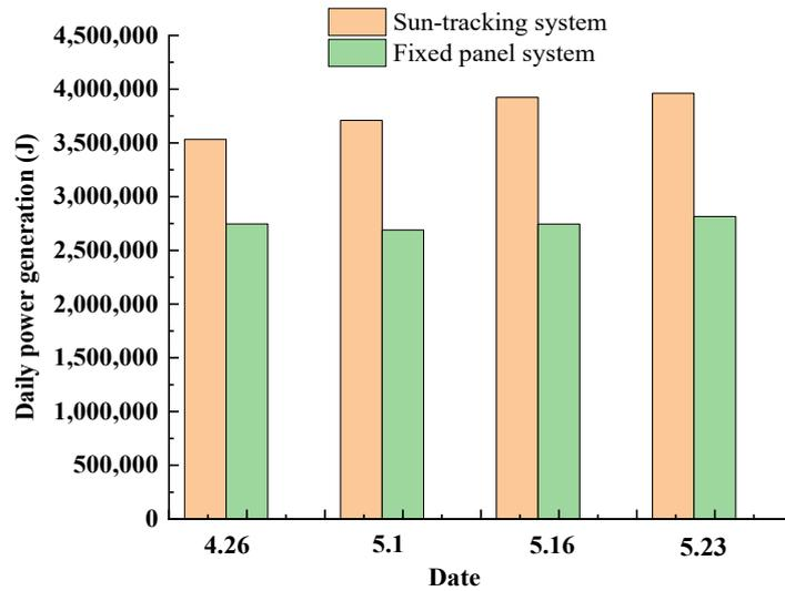
**Figure 7.** Comparisons on daily power output between the passive sun-tracking solar panel system and the fixed solar panel system at four sunny days.
