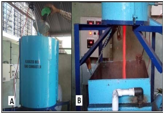
Figure 4. Fluidized bed combustor showing A) Loading and B) unloading of hot sand.
