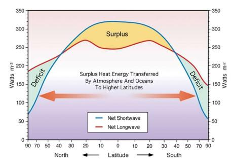
Figure 1. Heat energy transfer from surplus to deficit [13].
