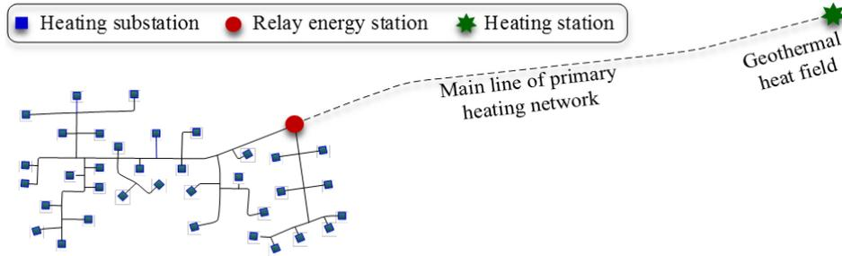
**Figure 2.** Topological graph of the primary network in the new low temperature sustainable central heating system.
