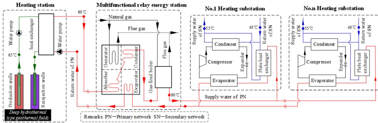
Figure 1. Sketch of the new low temperature sustainable central heating system.
