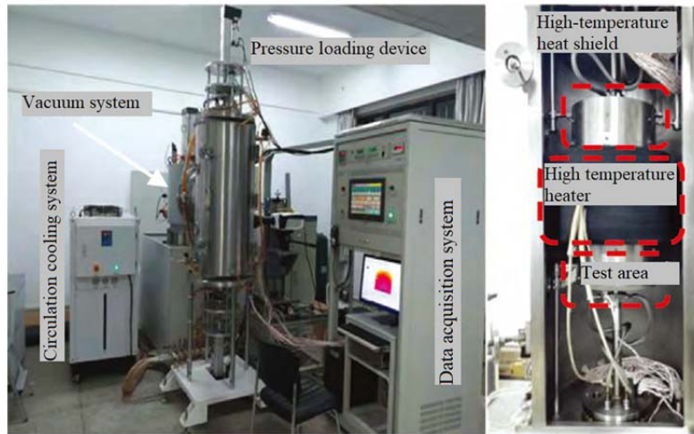
Figure 4. Test test system and high temperature vacuum test chamber internal diagram.
