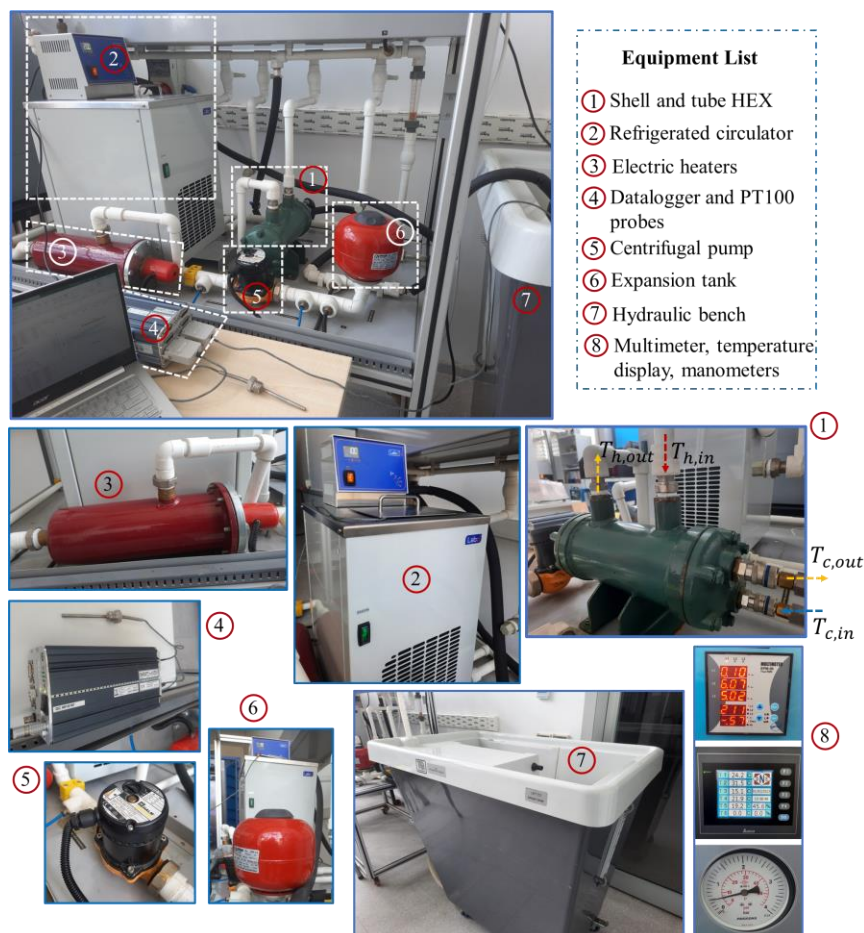
Figure 2. Experimental setup configuration and main components/devices.
