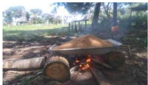
Figure 1. Rice husk carbonization process.
