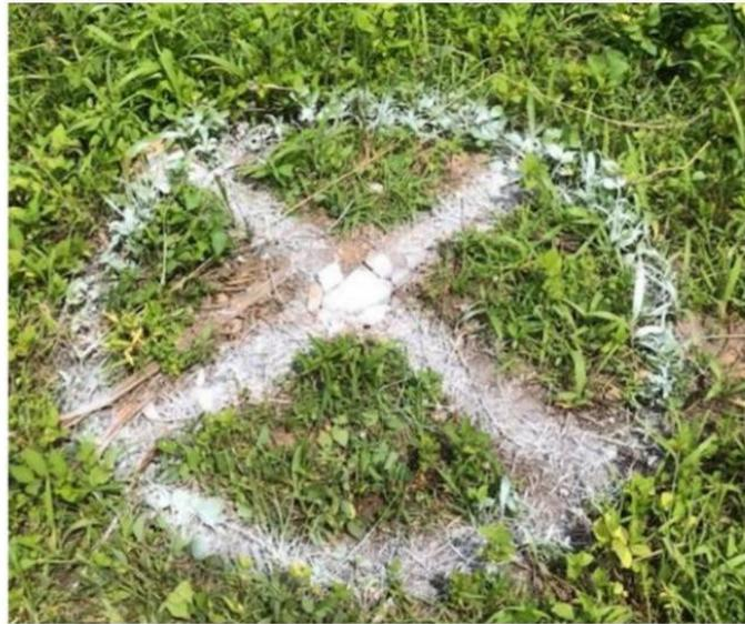
**Figure 2.** Sample ground control point (GCP) collected. The central point marked by the cross was collected using Differential Global Positioning System (DGPS) in the static observation method to ensure high accuracy.
