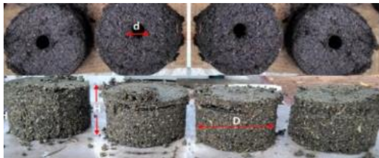
Figure 4. Briquette essential dimensions.
