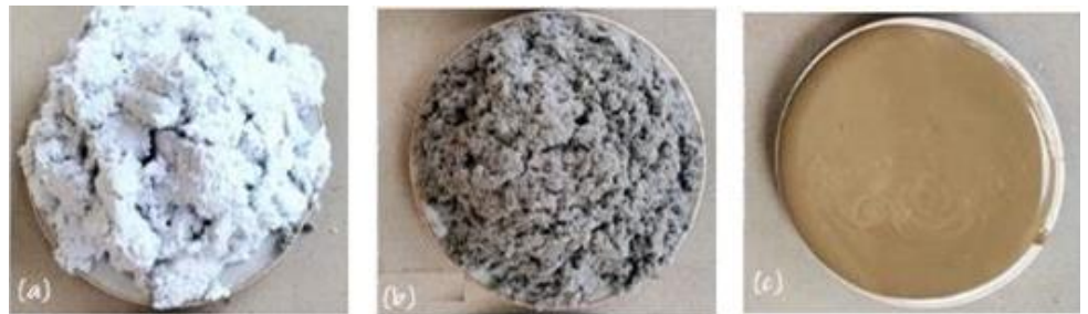
Figure 2. Samples of the three types of binder used in the experiment, (a) used printing paper pulp; (b) newsprint pulp; (c) clay suspension [28].
