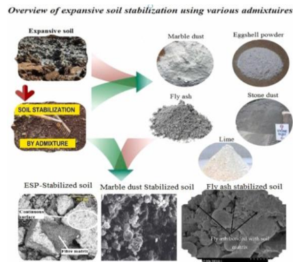
Figure 2. Procedures to evaluate soil suitability during stabilization [27].
