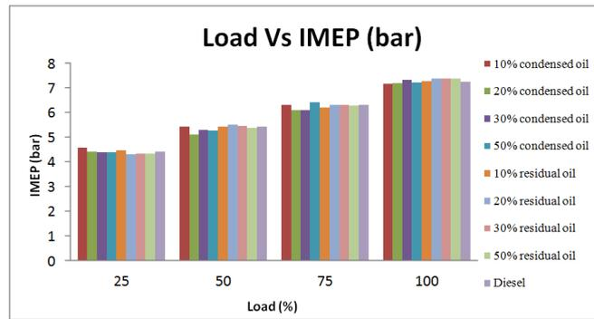
Figure 4. Indicated mean effective pressure at all loads.
