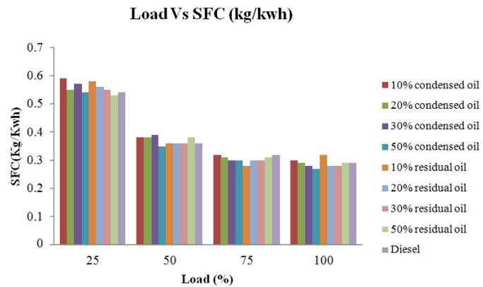
**Figure 7.** Specific fuel consumption for condensed and residual oil at all loads.
