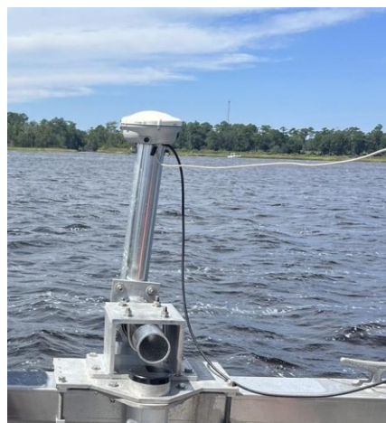
Figure 4. Echosounder acquisition survey setup, including pole-mounted Trimble R8s GPS receiver.
