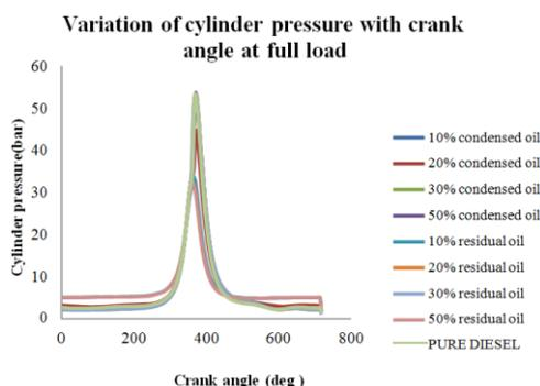
**Figure 8.** Variation of cylinder pressure with crank angle at full load.
