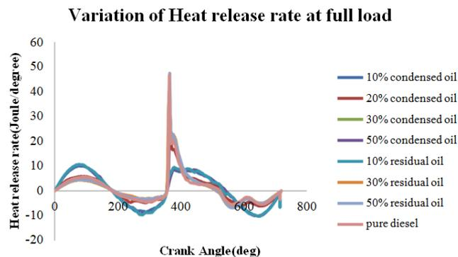
**Figure 10.** Heat release rate for condensed and residual oil at full load.
