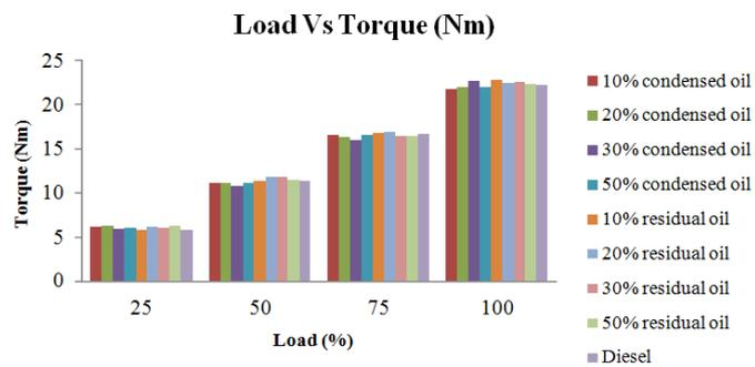
**Figure 6.** Torque for condensed and residual oil at all loads.
