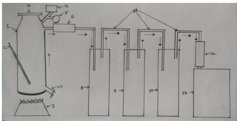
**Figure 1.** Experimental setup for pyrolysis of plastic waste.
