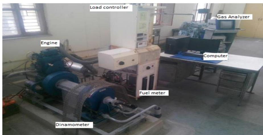
**Figure 2.** Experimental setup to study of combustion and performance efficiency of diesel engine.
