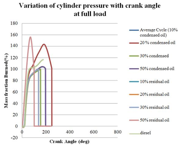
**Figure 9.** Variation of mass fraction burned with crank angle at full load.
