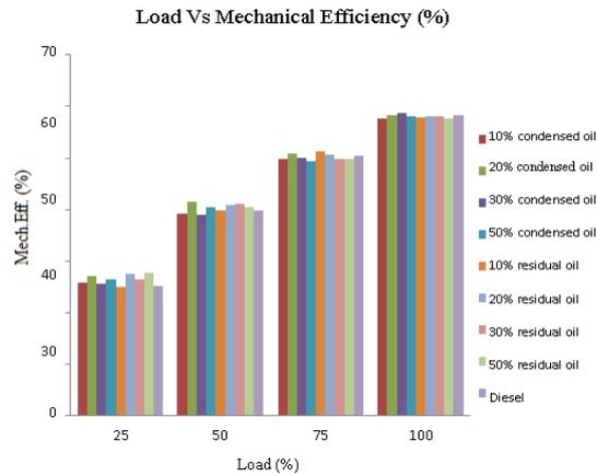
**Figure 3.** Mechanical efficiency of condensed and residual oil at all loads.
