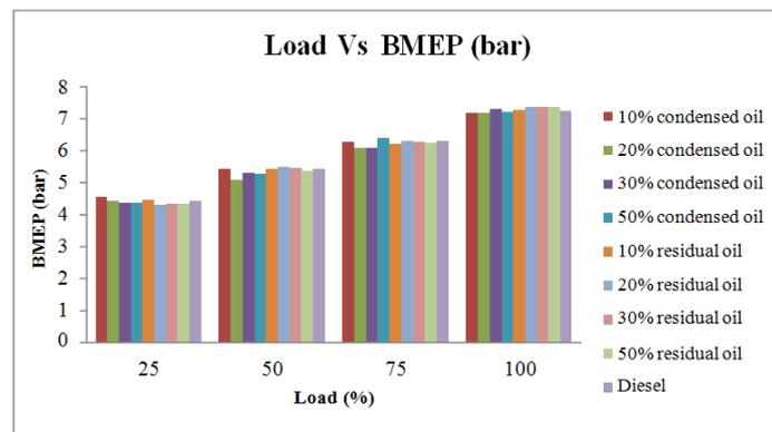
Figure 5. Brake mean effective pressure (BMEP) at all loads.
