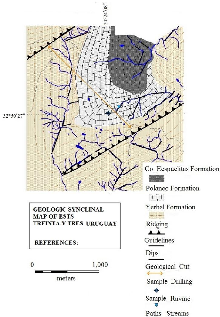
Figure 3. Geological map of Region I (East Syncline), Treinta y Tres.
