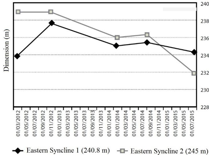
**Figure 17.** Water level graph in two wells of the East Syncline, Treinta y Tres.
