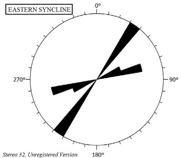
**Figure 6.** Lineament compass rose for Region I, East Syncline, Treinta y Tres. The N 35° to 45° E direction corresponds to the axis of the syncline, structure on which the Sinclinal del Este 1 borehole is developed, and to the thrusts indicated in the cartography. The direction N 60° to 70° E corresponds to faults of minor presence in the area.
