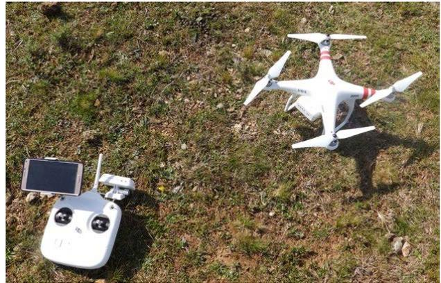
**Figure 2.** Unmanned aerial device (DJI DRONE–Phantom II Vision+).
