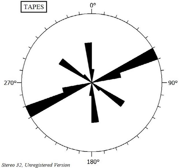
**Figure 13.** Lineament compass rose for Region II, Tapes Grande Syncline, Lavalleja.
