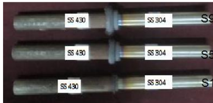
Figure 2; Samples of Friction welded joints.
