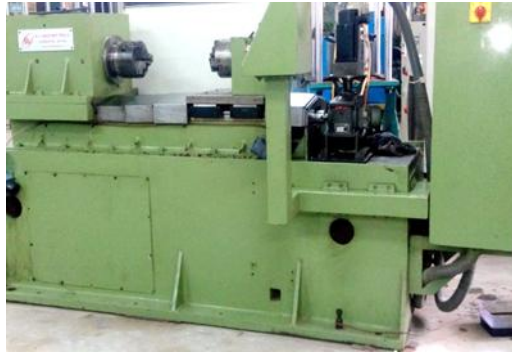
Figure 1; Photograph of Friction welding Machine.
