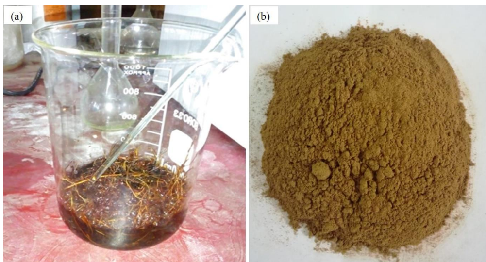
Figure 2. (a) Alkali treatment of coir fibre; (b) Alkali treated coir fibre powder.
