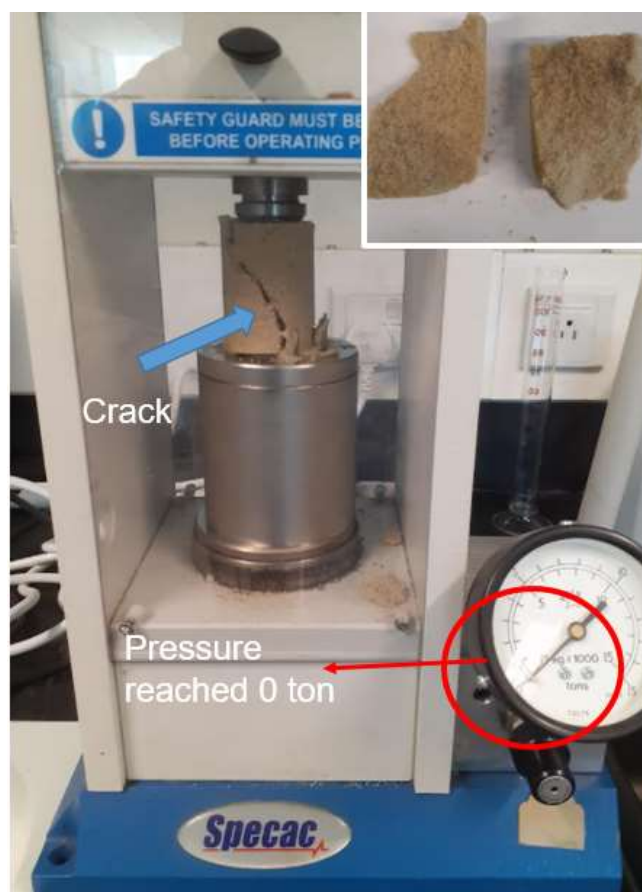
Figure 2. Compressibility test of the copolymer-reinforced cylindrical sand blocks. The inset shows the cracked block after the block is compressed.
