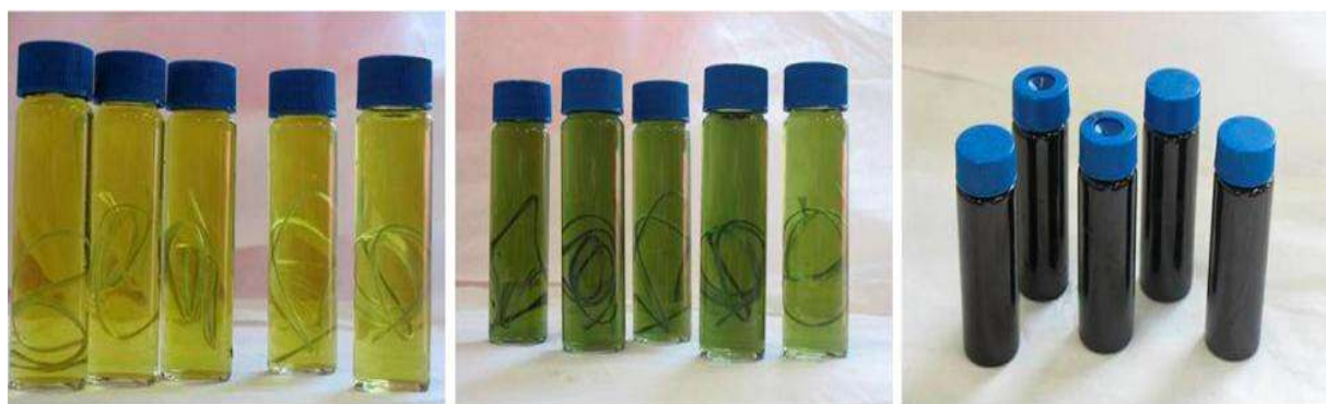
Figure 2. In-situ chemical polymerization by single bath process [59] .
