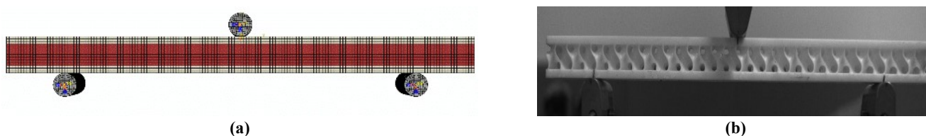
Figure 5. 3 Point bending (a) Abaqus model layout (b) experimental setup.
