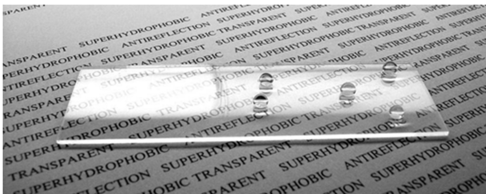
Figure 8. Photograph of the glass slide coated with superhydrophobic multilayer based on silica nanoparticles and poly(allylamine hydrochloride). Reproduced with permission from the American Chemical Society [169] .
