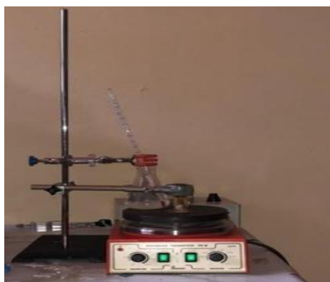
Figure 1. System consisting of a magnetic stirrer and thermometer, which allowed the sample to be homogenized and its temperature measured to control the variable.
