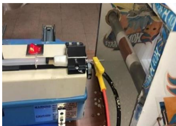
Figure 3. PVDF sample, with DMF/MEC as the solvent, inside the syringe, ready to begin the electrospinning technique.
