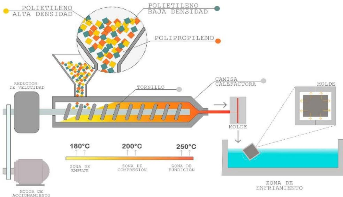
**Figure 1.** Plastic extrusion-pressure (injection) process.
