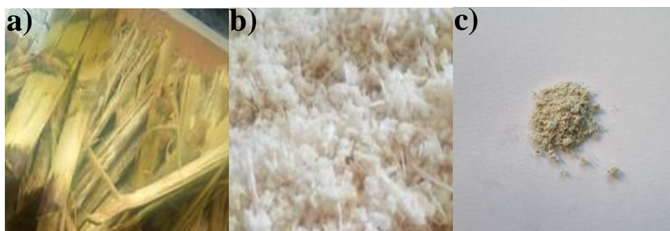
Figure 1. (a) Photographs showing the sugarcane bagasse biomass; (b) washed and pulverized biomass; (c) biomass ash.
