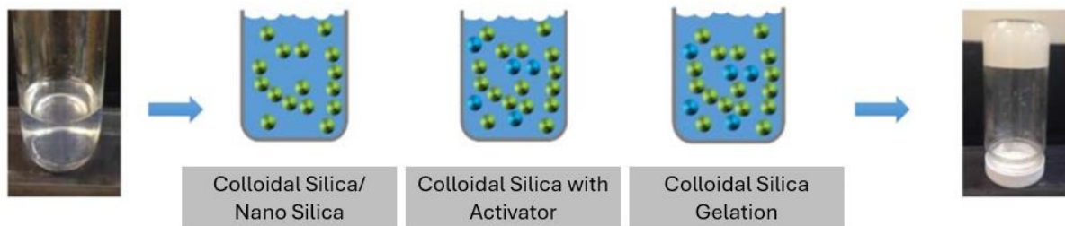
Figure 10. Schematic illustration of gelation of nano silica system [94].
