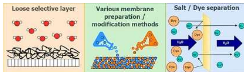
Figure 1. Polyester membrane for water purification by desalination and dye removal [31]. Reproduced with permission from Elsevier.
